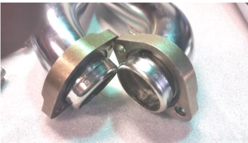
Fig. 2.1 Install both flanges and retaining rings
