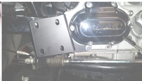
Fig. 2.2 Install mounting bracket
