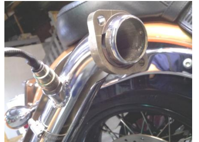
Fig 1.3 install flange, ring and sensor
