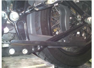
Fig 1.2 install left side bracket MBK-S110
