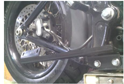
Fig 1.1 install right side bracket MBK-S111
