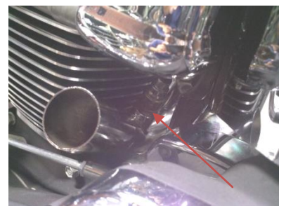
Fig 1.5 install crossover pipe first, then install O2 sensor.
