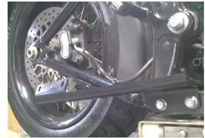
Fig 1.1 install right side bracket MBK-S111
