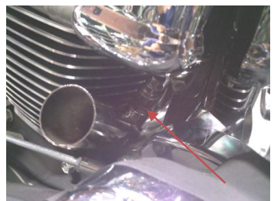
Fig 1.5 install crossover pipe first, then install O2 sensor.
