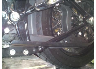
Fig 1.2 install left side bracket MBK-S110
