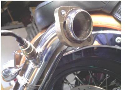
Fig 1.3 install flange, ring and sensor
