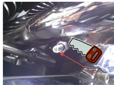
Fig 1.9 tighten T-bolt clamp and if you wish cut the end of the bolt threads flush with the nut
