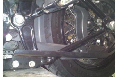
Fig 1.2 install left side bracket MBK-S110
