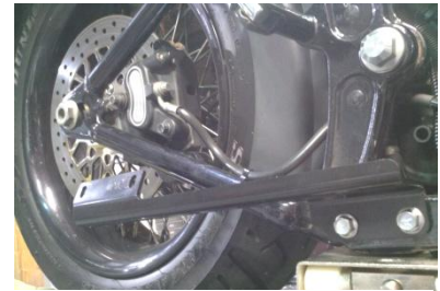
Fig 1.1 install right side bracket MBK-S111
