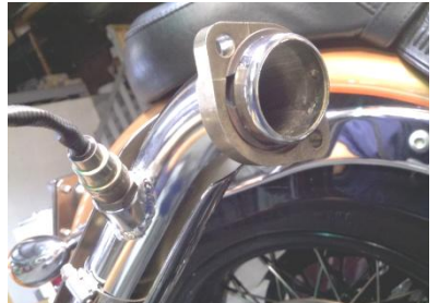
Fig 1.3 install flange and retaining ring
