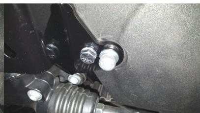
Figure 2.8 install bracket use new 3/8" split washer discard stock.
