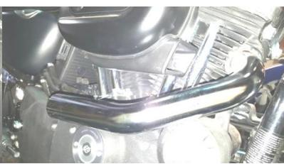
Figure 2.10 Install front pipe.
