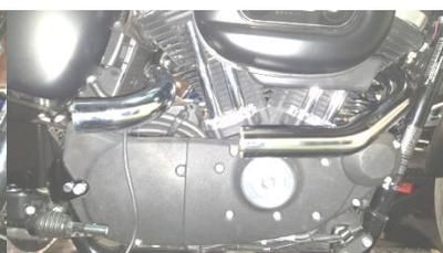
Figure 2.11 Install rear pipe.
