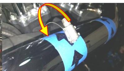
Figure 2.18 Arrow indicates direction of clamp insertion.
