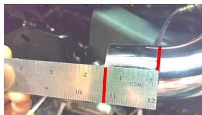
Figure 2.13 Mark a line @ 1-3/8" from edge of pipes.
