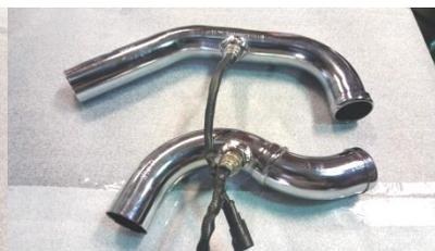
Figure 2.3 Install 18mm sensors.
