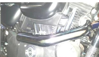
Figure 2.10 Install front pipe.
