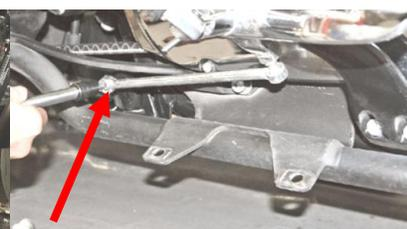
Figure 2.20 Re-install brake rod as it was prior to installation.
