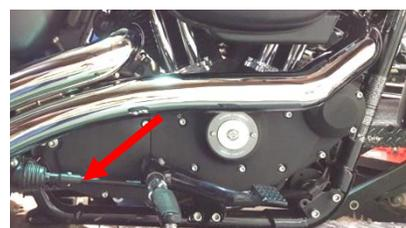
Figure 2.21 Install brake rod and controls.
