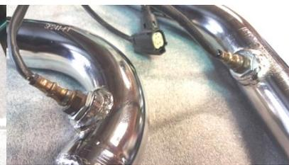
Figure 2.4 Install 12mm sensors.
