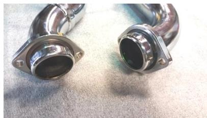
Figure 2.5 install retaining rings and flanges.
