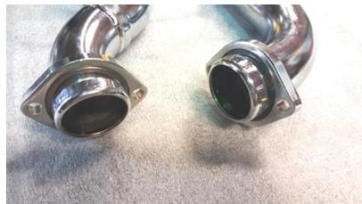
Figure 2.5 install retaining rings and flanges.
