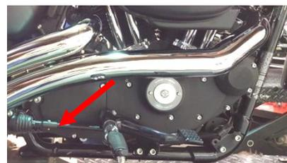
Figure 2.21 Install brake rod and controls.
