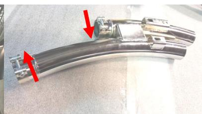
Figure 2.12 Insert (2) barrel clamps note direction of head screw.
