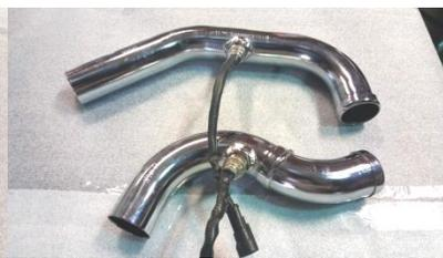
Figure 2.3 Install 18mm sensors.
