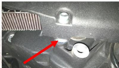
Figure 2.7 Washer installed as spacer.
