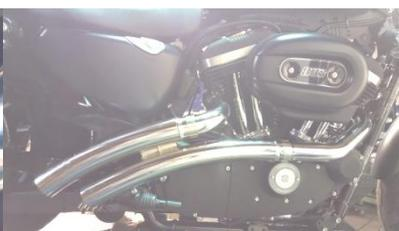
Figure 2.14 Install muffler assembly
