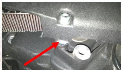
Figure 2.7 Washer installed as spacer.
