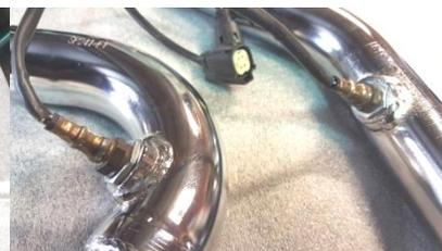
Figure 2.4 Install 12mm sensors.
