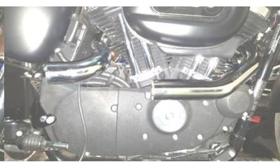
Figure 2.11 Install rear pipe.
