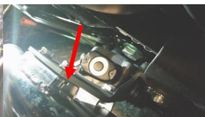
Figure 2.15 Mounting bracket and welded brackets are flush at edge.
