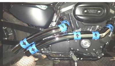
Figure 2.19 Install rear shield.
