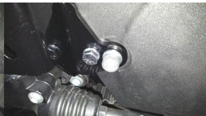
Figure 2.8 install bracket use new 3/8" split washer discard stock.
