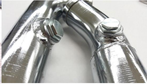
Figure 2.5 install adapter and plug.
