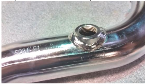
Figure 2.2 install adapter and plug
