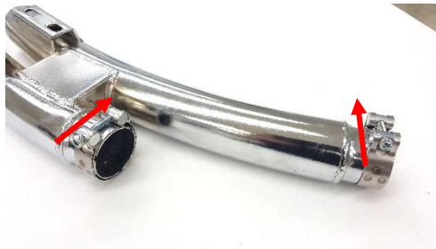
Figure 2.7 insert barrel clamps note screw head direction.
