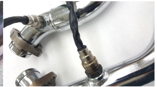
Figure 2.3 install O2 sensor
