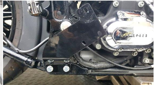
Figure 2.6 install mounting bracket.
