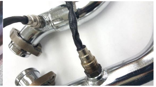
Figure 2.3 install O2 sensor
