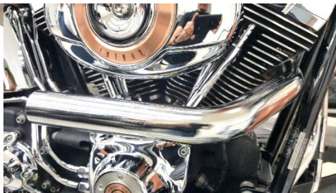
Figure 2.8 install front pipe.
