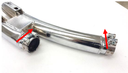
Figure 2.7 insert barrel clamps note screw head direction.
