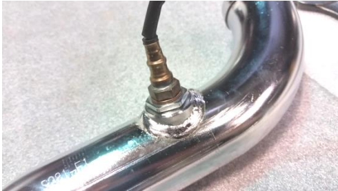
Fig 2.4 install adapter then 12mm sensor
