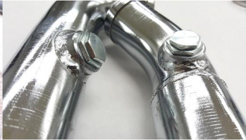
Figure 2.5 install adapter and plug.
