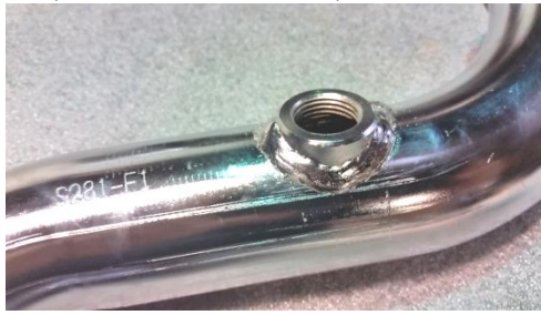
Figure 2.2 install adapter and plug
