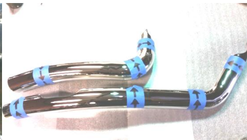
Fig. 2.11 Arrows indicate direction of hose clamp insertion
