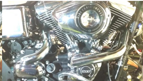
Fig.2.8 Install rear header using stock flange nuts and 1/2" socket
