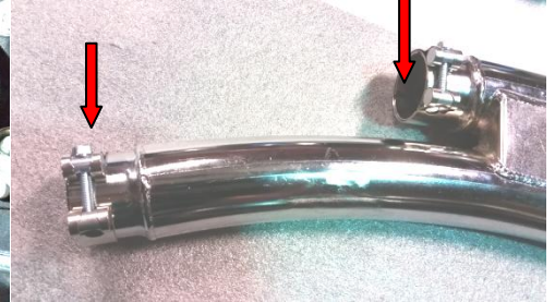
Fig. 2.6 Insert barrel band clamps over the muffer inlets as shown arrow indicates screw direction
