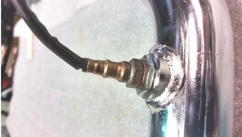
Fig. 2.4 Install 12mm sensor fist install adapter from M18 to M12
