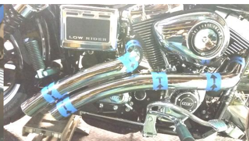
Fig. 2.14 Install rear heat shield
