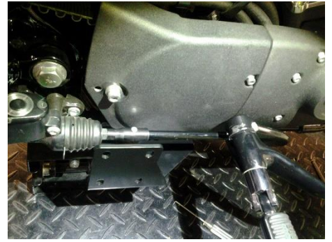
Figure 2.3 re-install brake rod using pin and retaining ring
