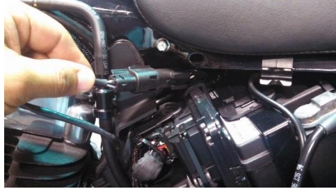
Fig. 1.5 disengage sensor harness
