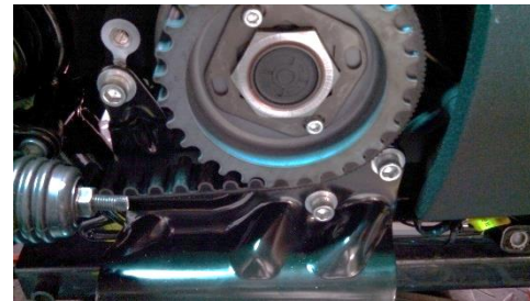
Fig. 1.11 remove mounting bar/bracket
