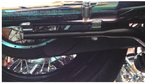
Fig. 1.2 remove bolts holding mufflers
