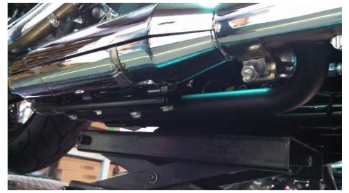
Fig. 1.3 remove bolts holding mufflers
