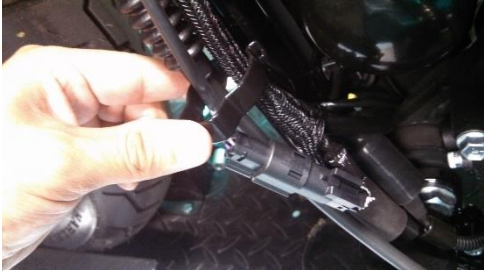
Fig. 1.4 disengage sensor harness
