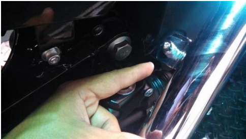
Fig. 1.7 loosen muffer clamps
