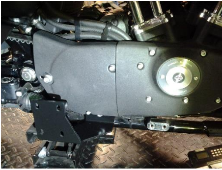
Figure 2.2 re-install belt cover
