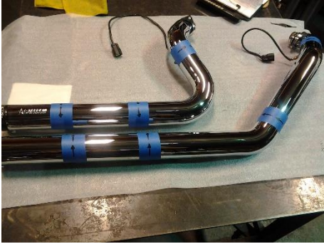
Figure 2.4 mark center on heat shield clips over painter's tape
