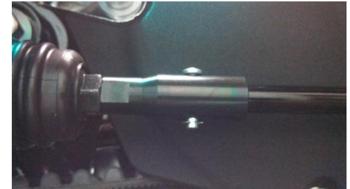
Fig. 1.9 remove retaining ring and pin
