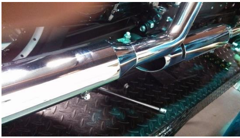
Fig. 1.1 loosen muffer clamps
