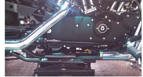
Fig. 1.6 loosen muffer clamps
