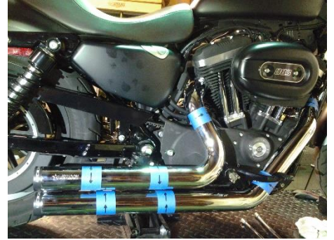
Figure 2.6 install rear pipe assembly
