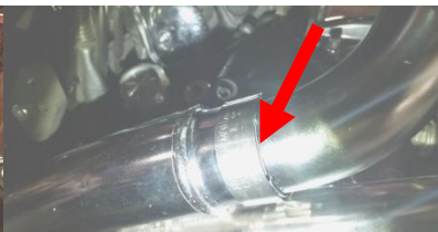
Figure 2.17 install rear heat shield.
