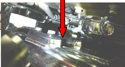
Figure 2.11 Insert back plate brackets as shown.
