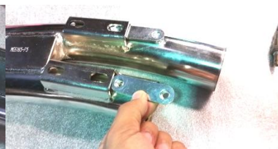
Figure 2.10 Install barrel band clamps as shown.
