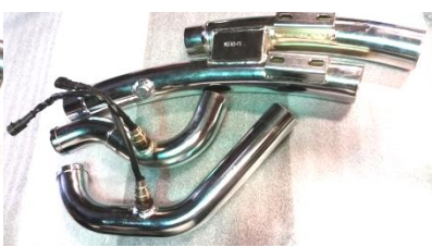
Figure 2.6 (07-09) Install 18mm sensors and plug muffler.
