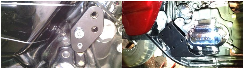
Figure 2.2 Install peg raiser as shown.
