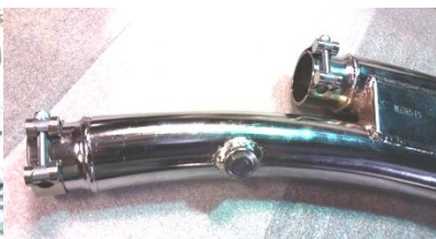
Figure 2.9 Install rear header and align it with front header.
