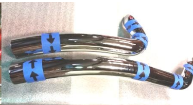
Figure 2.13 Align headers with muffler as shown.
