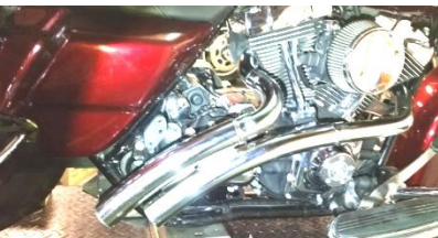
Figure 2.12 Front of brackets welded on muffler are flush with mounting bracket.
