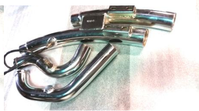
Figure 2.7 (10-up) Install 12mm sensors and plug front head pipe.
