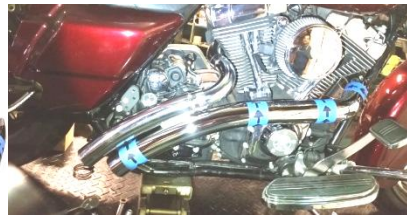
Figure 2.14 Mark arrows and center of welded clips as shown.
