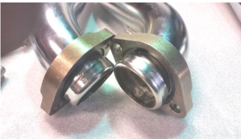
Figure 2.1 install flange and retaining clip
