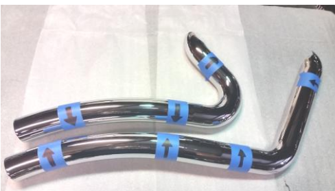
Figure 2.10 mark center and direction
