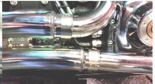
Figure 2.9 headers go inside about 1-3/8"
