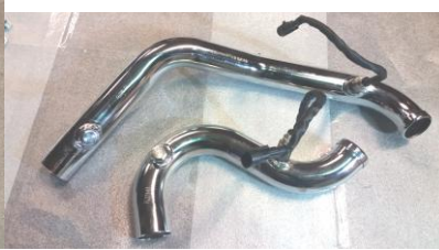
Figure 2.6 (07-09) Install 18mm sensors and 12mm plugs.
