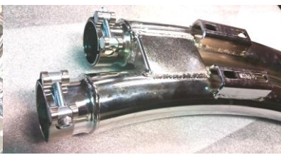
Figure 2.10 Install barrel band clamps as shown.
