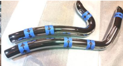
Figure 2.14 Mark arrows and center of welded clips as shown.
