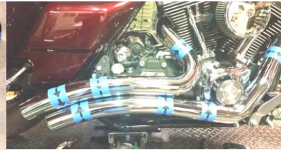
Figure 2.15 Install front shield use a 5/16 inch nut driver.
