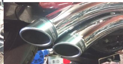
Figure 2.20 Install end caps use some type of locking glue.
