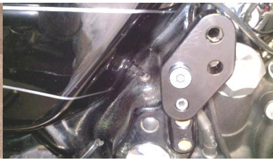
Figure 2.2 Install peg raiser as shown.
