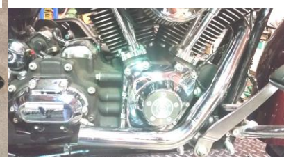
Figure 2.8 Install front header using stock flange nuts.
