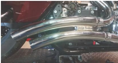
Figure 2.13 Align headers with muffler as shown.
