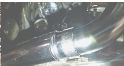
Figure 2.18 make sure barrel clamps are flush with the front of slotted inlets for a tight seal.
