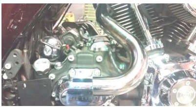
Figure 2.9 Install rear headers and align it with front header.
