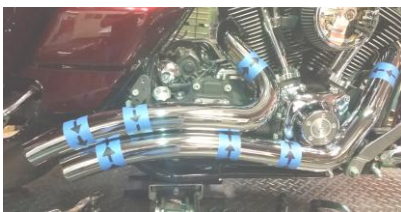
Figure 2.17 install rear heat shield.
