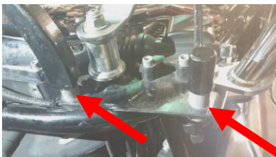
Models (95-08) use bigger screws and spacers as shown
