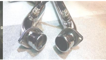
Figure 2.4 Install retaining rings and flanges.
