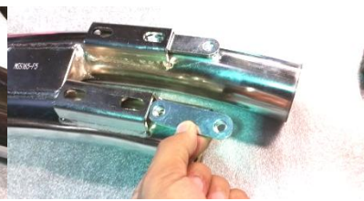
Figure 2.11 Insert back plate brackets as shown.
