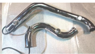
Figure 2.7 (10-up) Install 12mm sensors and 18mm plugs.
