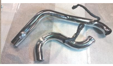
Figure 2.6 (07-09) Install 18mm sensors and 12mm plugs.
