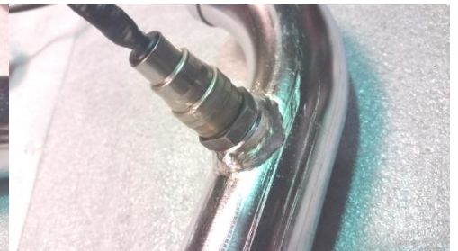
Fig. 2.3 Install M18 sensors use a 7/8" or M22 wrench
