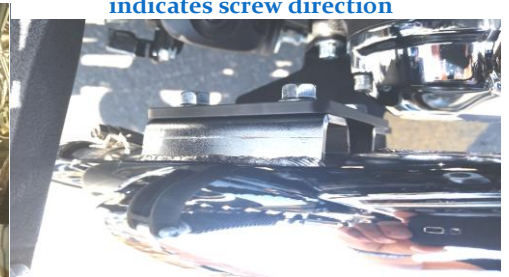
Fig.2.9 Install muffler as shown brackets must be flush use a 1/2" wrench
