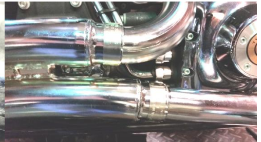
Figure 2.9 headers go inside about 1-3/8"
