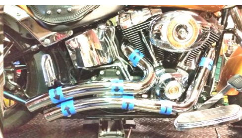
Figure 2.14 install rear heat shield and secure it with hose clamps
