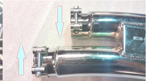
Figure 2.6 install barrel band clamps
