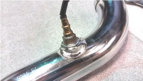
Fig 2.4 install adapter then 12mm sensor
