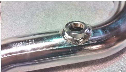
Figure 2.2 install adapter and plug
