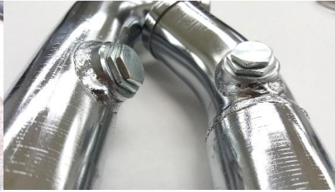
Figure 2.5 install adapter and plug.
