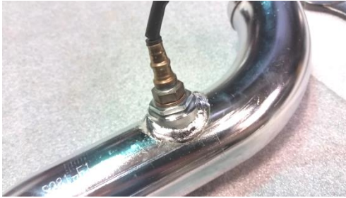
Fig 2.4 install adapter then 12mm sensor
