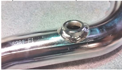
Figure 2.2 install adapter and plug
