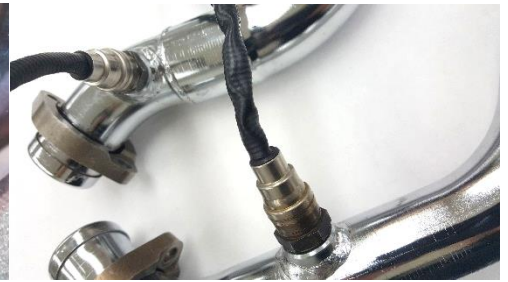
Figure 2.3 install O2 sensor
