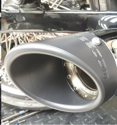
Fig. 2.17 Install system end cap. This end cap can also be rotated every 30°
