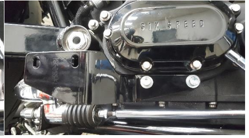
Fig. 2.3 Install mounting bracket.
