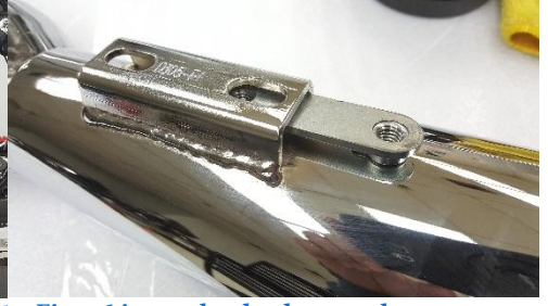
Fig.2.6 insert back-plate as shown.
