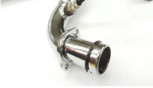
Fig. 2.4 Install flanges and retaining rings.
