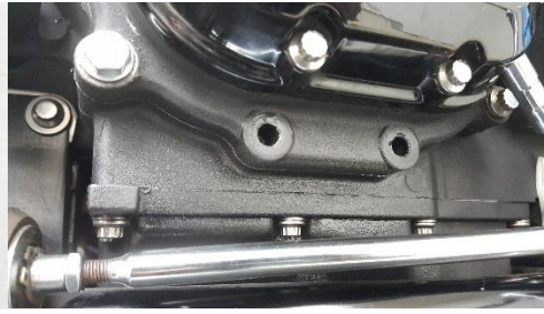
Fig. 2.2 Remove 2 screws as shown.
