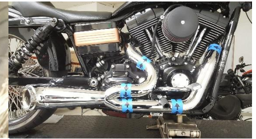
Fig. 2.12 Install rear heat shield.
