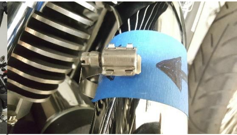
Fig. 2.11 arrow indicates the direction of hose clamp insertion.
