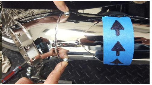
Fig. 2.15 tip of heat shield must be located between the two screws as shown
