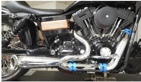
Fig. 2.10 install front heat shield.
