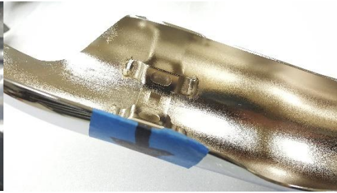
Fig. 2.8 clip welded inside heat shield.
