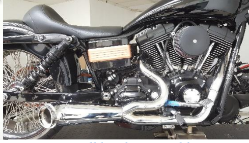
Fig.2.5 Install header assembly, use stock flange nuts.
