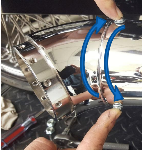
Fig. 2.16 Note: you can rotate both the turn-out (elbow) any direction you want by removing the 3 screws holding it to the muffler
