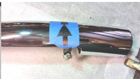
Figure 2.11 install hose clamps only one on each heat shield at the end (#28)
