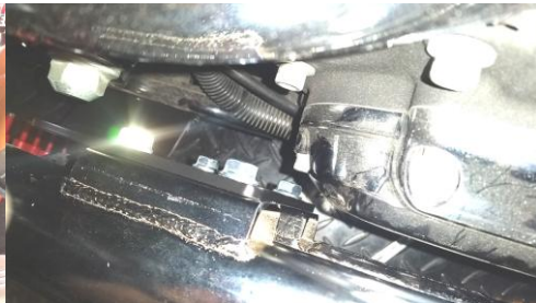
Figure 2.8 front of brackets align flush
