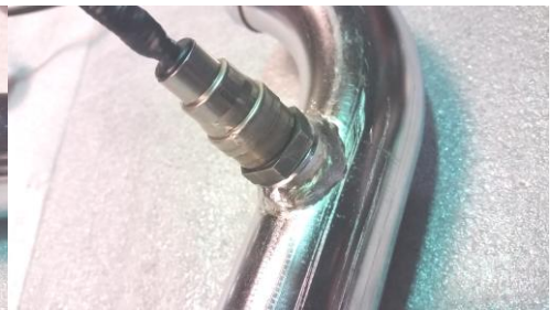
Figure 2.3 install O2 sensor
