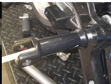
Fig. 1.18 remove peg bracket
