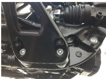
Fig. 3.6 remove mid control screws
