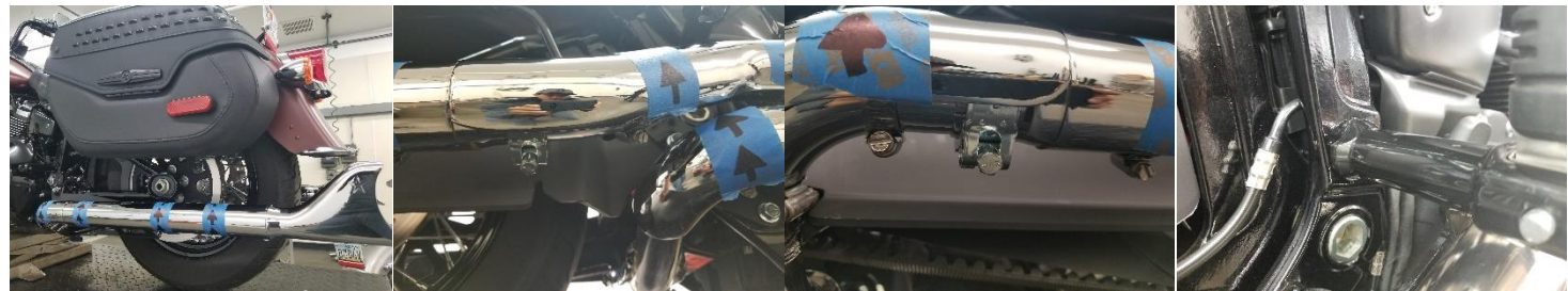
Fig. 5.33 install rear heat shield
