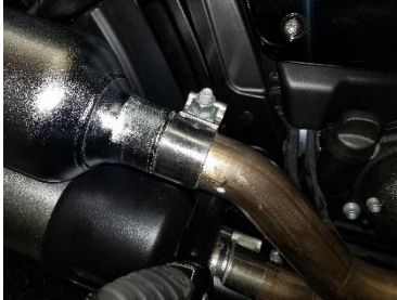
Fig 1.5 loosen muffer clamps
