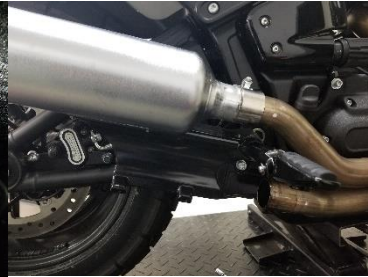
Fig. 1.7 remove upper muffer.
