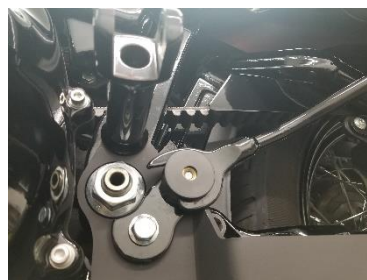
Fig. 5.13 install left side saddle bracket
