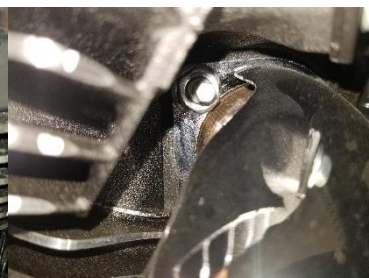
Fig. 3.9 remove front flange nuts
