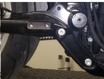
Fig. 2.11 remove mounting bracket
