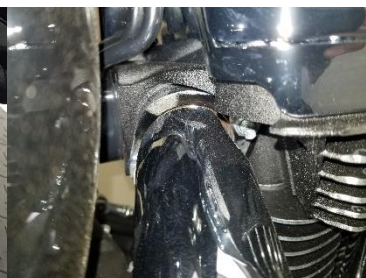
Fig. 3.8 remove rear flange nuts
