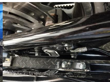
Fig. 3.1 remove upper muffler screws
