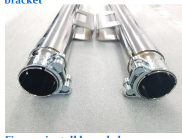
Fig. 5.17 install barrel clamps.
