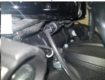
Fig. 2.7 disconnect rear sensor
