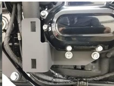
Fig. 5.4 install transmission bracket
