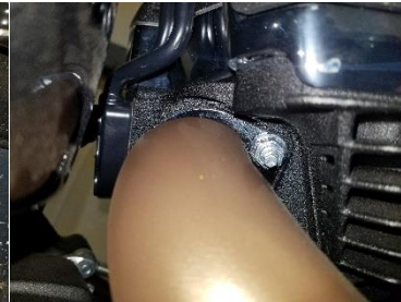
Fig. 1.11 remove rear flange nuts
