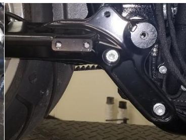
Fig. 1.19 remove mounting bracket
