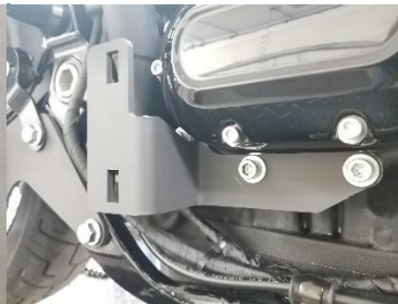
Fig. 5.3 install transmission bracket
