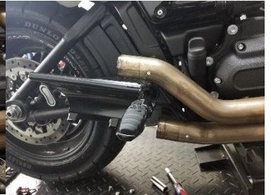
Fig. 1.8 remove lower muffer
