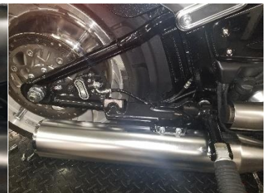
Fig. 2.5 remove upper muffer
