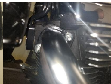
Fig. 2.9 remove rear flange nuts
