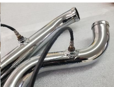
Fig. 5.15 install O2 stock sensors
