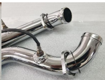
Fig. 5.16 install rings and flanges
