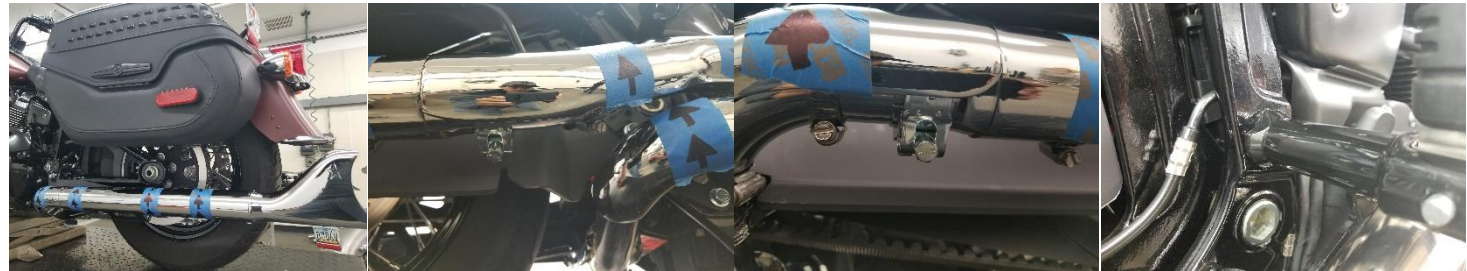
Fig. 5.33 install rear heat shield
