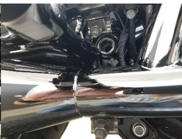
Fig. 3.3 loosen both muffler clamps
