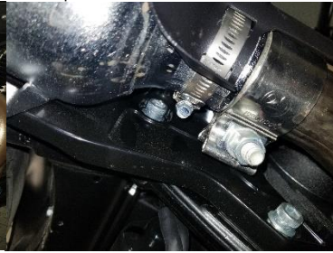
Fig. 1.3 remove hose clamps
