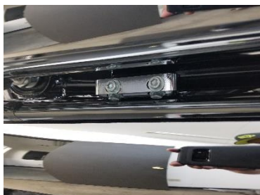
Fig. 3.2 remove lower muffler screws
