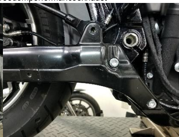
Fig. 4.7 remove bracket screws
