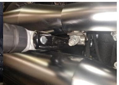
Fig. 2.1 loosen upper clamp
