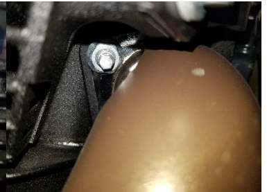
Fig. 1.12 remove front flange nuts
