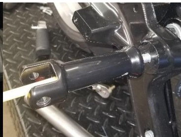
Fig. 1.18 remove peg bracket
