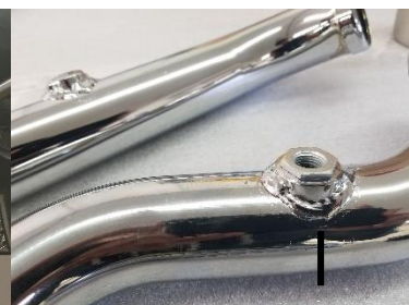
Fig. 5.14 install O2 adapters
