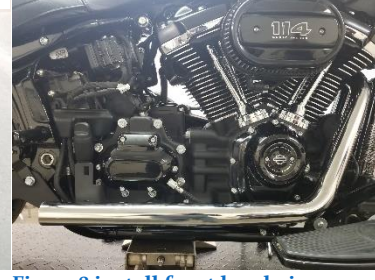
Fig. 5.18 install front head pipe
