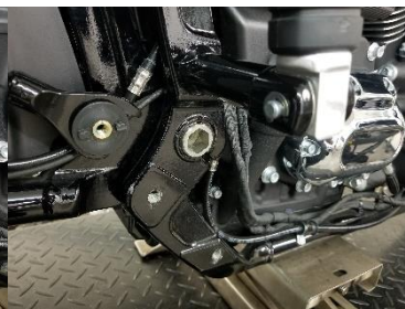
Fig. 4.8 remove mounting bracket
