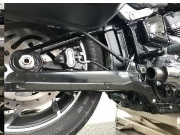
Fig. 4.4 remove slip-on muffler
