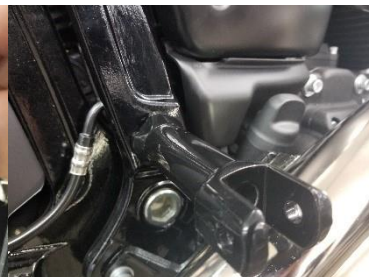
Fig. 5.28 install peg right side
