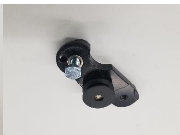
Fig 5.10 passenger peg with stock saddlebag hardware L/S
