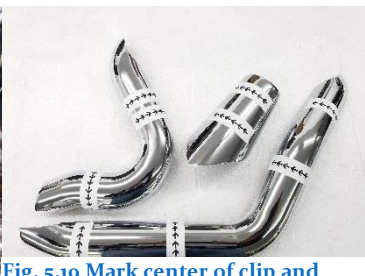
Fig 5.19 Mark center of clip and direction of clamp insertion
