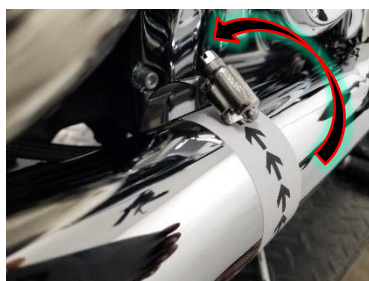
Fig. 5.21 arrow indicate direction of insertion
