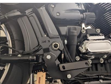
Fig 5.3 Saddlebag relocater bracket wide tire models.
