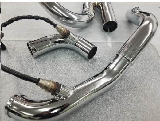
Figure 2.5 Install O2 sensors (07-09).
