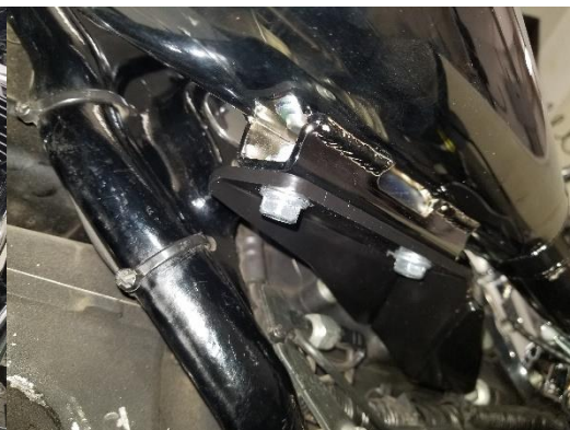
Figure 2.12 attach bracket to mounting bracket flush or a (+/-) 1/8"
