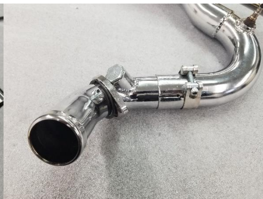
Figure 2.9 insert rear pipe in curved pipe on muffler/pipe assembly.
