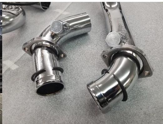
Figure 2.3 Install retaining rings & flanges/ install plugs (95-06) (09-16)
