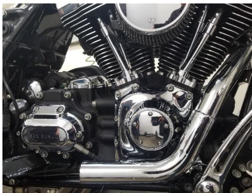
Figure 2.7 Install front header pipe.
