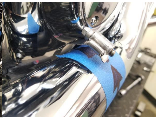
Figure 2.15 insertion of clamp arrow indicates direction of insertion.
