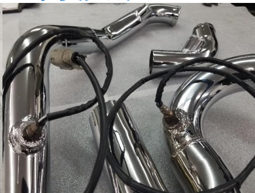
Figure 2.6 Install O2 sensors (09-17).
