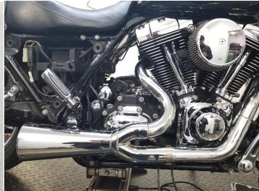
Figure 2.11 Install muffler/pipe assembly.
