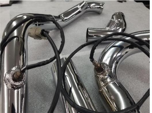
Figure 2.6 Install O2 sensors (09-17).
