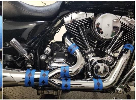
Figure 2.18 Install collector shield.
