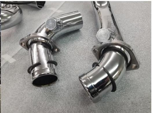
Figure 2.3 Install retaining rings & flanges/ install plugs (95-06) (09-16)
