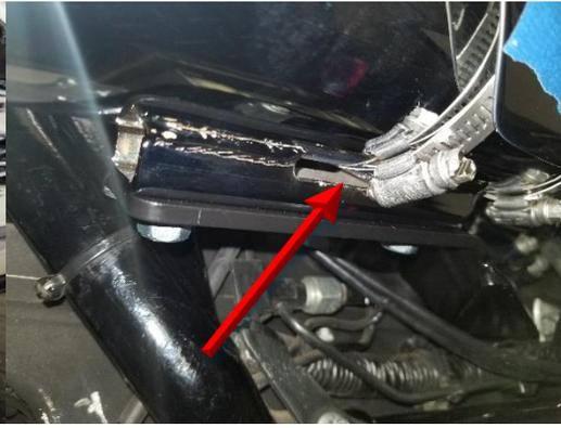
Figure 2.20 clamp goes thru welded bracket.
