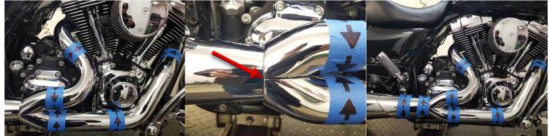
Figure 2.16 Install rear shield.
