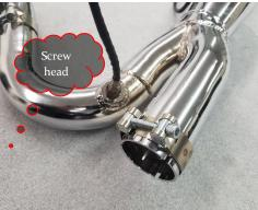
Figure 2.10 insert barrel clamp as shown
