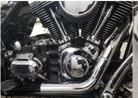
Figure 2.7 Install front header pipe.
