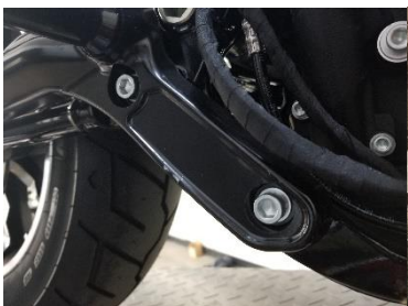
Fig. 3.10 remove mounting bracket
