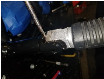
Fig. 1.17 pull pin and remove peg
