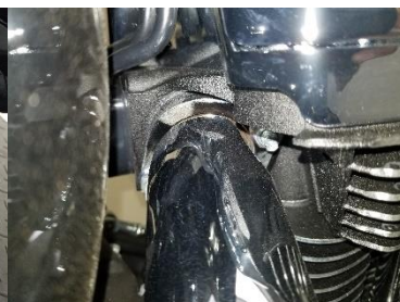
Fig. 3.8 remove rear flange nuts
