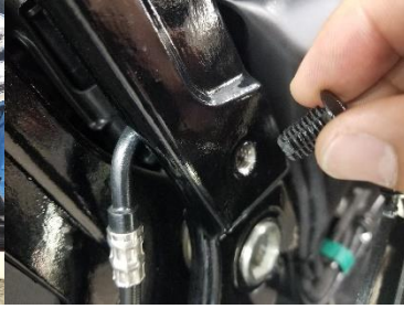
Fig. 5.22 remove plastic plug from thread hole on frame
