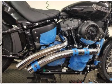
Fig. 5.18 install front heat shield
