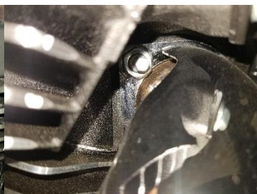
Fig. 3.9 remove front flange nuts
