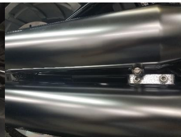
Fig. 2.3 remove screws upper muffer
