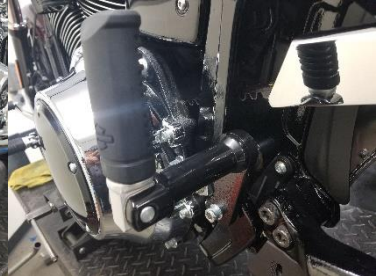
Fig. 5.28 install peg left side
