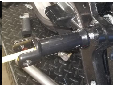
Fig. 1.18 remove peg bracket
