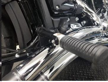
Fig. 5.27 install peg right side
