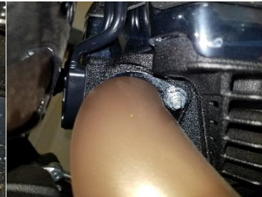
Fig. 1.11 remove rear flange nuts
