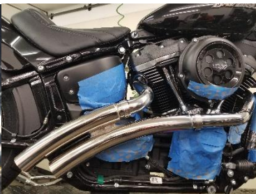
Fig. 5.15 install muffler assembly
