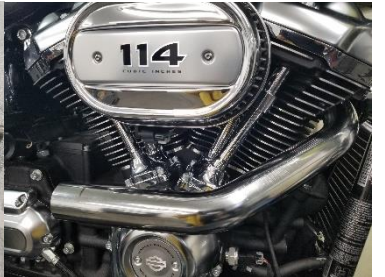
Fig. 5.12 install front pipe
