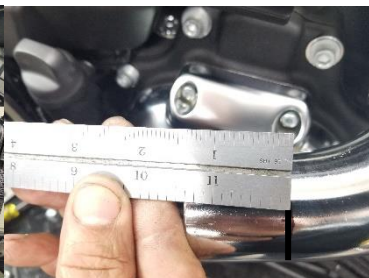
Fig. 5.14 mark a line @ 1-3/8" (35mm)
