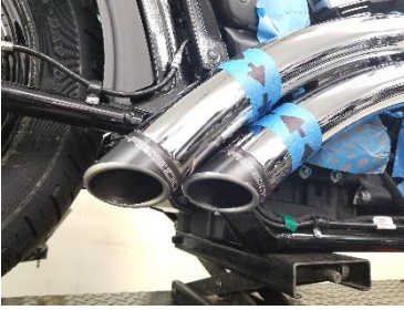
Fig. 5.21 install end caps
