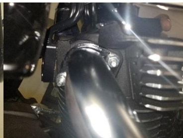
Fig. 2.9 remove rear flange nuts
