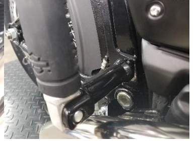
Fig. 5.24 reinstall peg on bracket.
