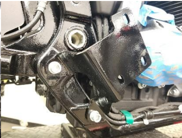
Fig. 5.3 install bracket slim tire
