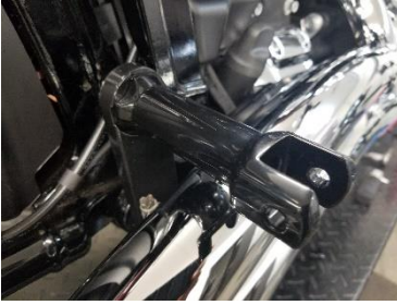
Fig. 5.25 wide tire bracket installation on right side
