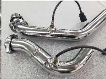
Fig. 5.10 install Oxygen sensors
