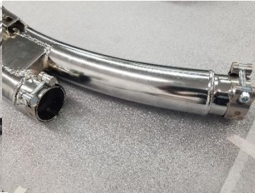
Fig. 5.11 insert barrel band clamps
