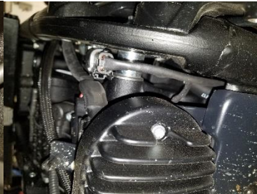
Fig. 1.10 locate front sensor
