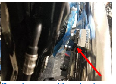
Fig. 5.16 secure muffler to bracket make brackets are flush to each other
