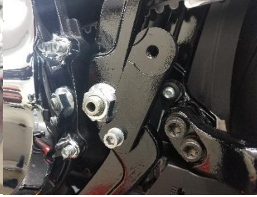
Fig. 5.26 wide tire bracket installation on left side
