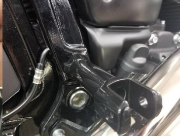
Fig. 5.23 install peg bracket
