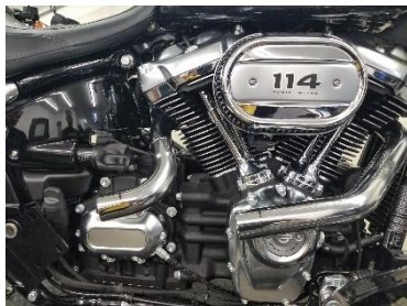
Fig. 5.13 install rear pipe
