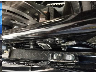
Fig. 3.1 remove upper muffler screws
