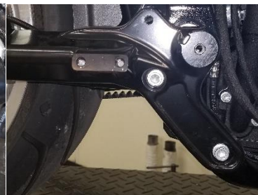
Fig. 1.19 remove mounting bracket
