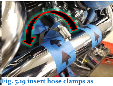
Fig. 5.19 insert hose clamps as shown
