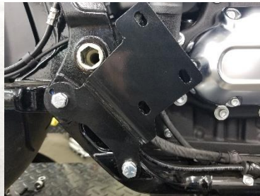
Fig. 5.2 install bracket wide tire
