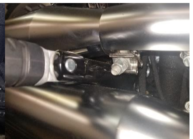
Fig. 2.1 loosen upper clamp
