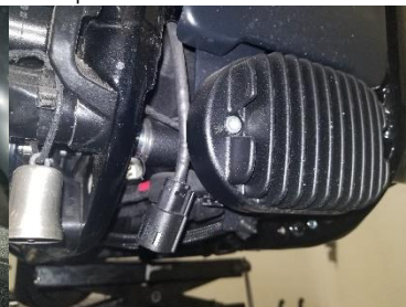
Fig. 2.8 disconnect front sensor
