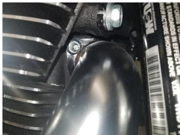
Fig. 2.10 remove front flange nuts
