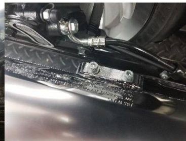
Fig. 2.3 remove screws upper muffer
