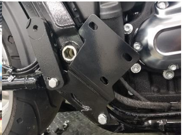
Fig. 5.4 wide tire right peg relocater
