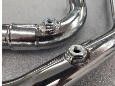
Fig. 5.9 install sensors adapters
