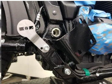
Fig. 5.7 saddle bag bracket support
