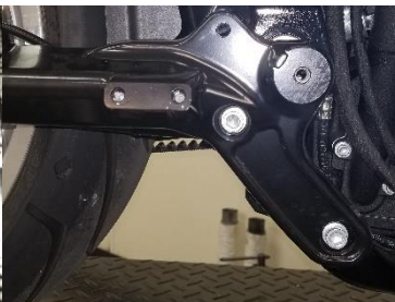
Fig. 2.11 remove mounting bracket
