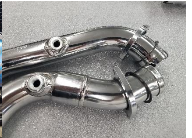
Fig. 5.8 install rings and flanges
