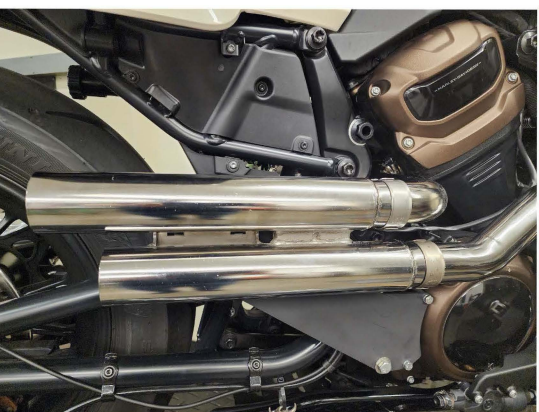
Fig.2.11 put in muffler as shown with the clamps on.
