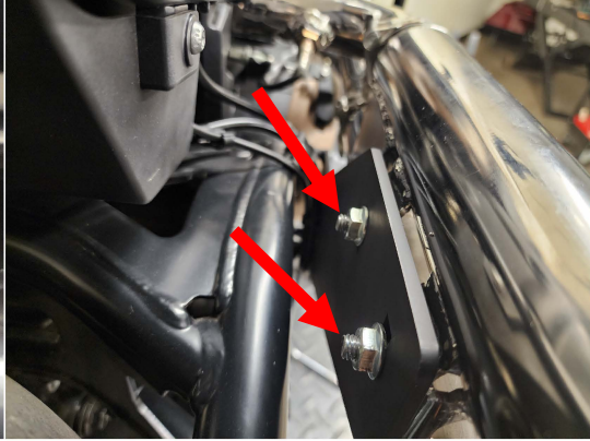
Fig.2.14 make sure to have the nuts on the back of the mounting bracket.
