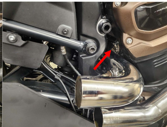
Fig.2.9 Install rear header pipe as shown screwed in correctly.
