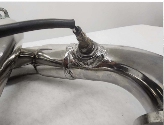
Fig.2.7 put in the O2 sensors as shown into the header pipes.
