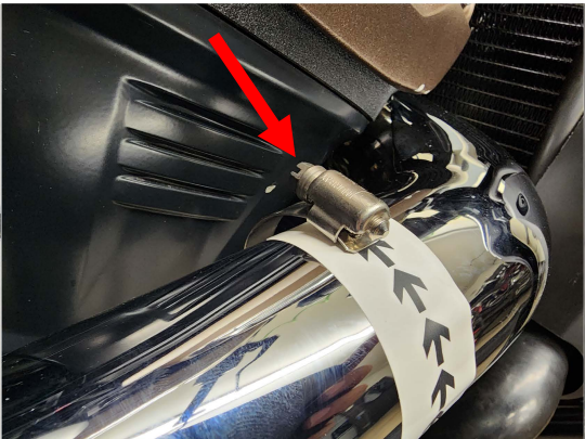
Fig.2.17 make sure worm clamp is inserted as shown above when installing this rear heatshield
