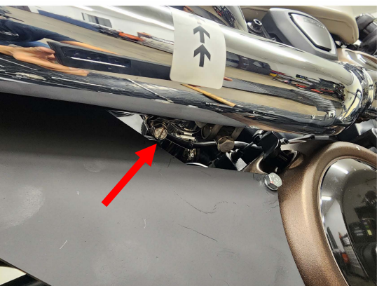
Fig.2.19 Make sure all worm clamps are tightened to the pipe where they do not fall.
