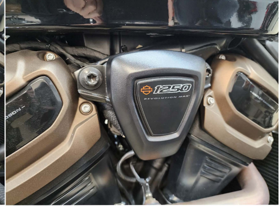
Fig.1.15 locate plastic emblem and remove
