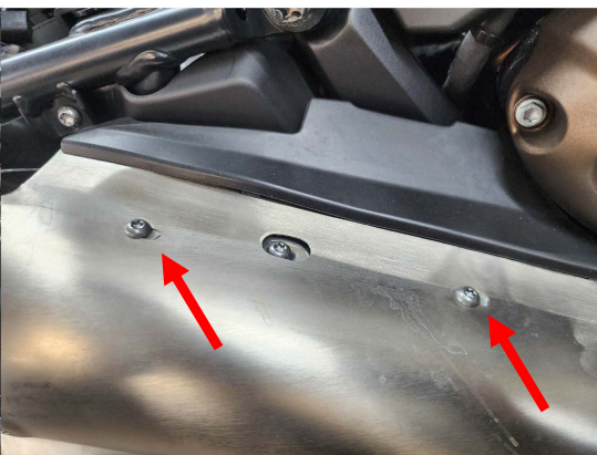
Fig.1.11 Locate these two top screws and remove them
