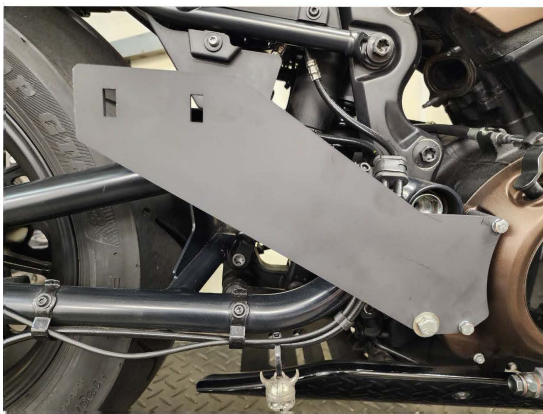
Fig.2.4 Once mounting bracket is put in it should look like this.
