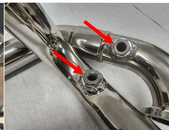
Fig.2.6 put in O2 adapters if needed into O2 holes.
