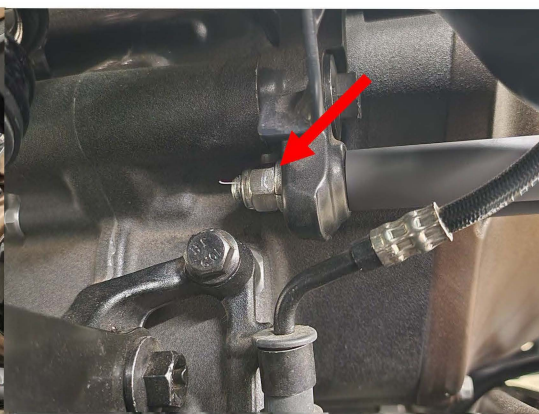
Fig.2.5 Dont forget to have the nut holding onto the screws for this bracket.
