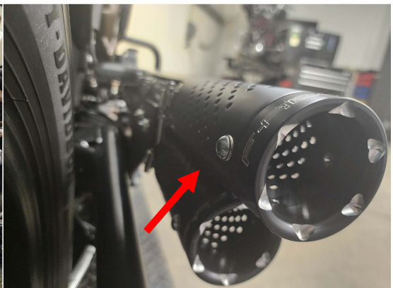
Fig.2.21 If you have end-caps you must screw them on as shown and that should be all for this installation.
