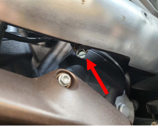
Fig.1.13 locate screw holding worm clamp and remove clamp and heat shield..
