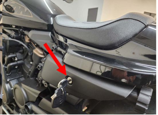
Fig.1.3 Insert key to remove the seat
