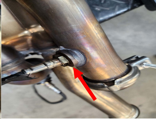
Fig.1.26 remove the O2 sensor attached to the front pipe.
