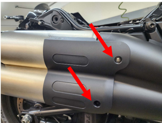
Fig.1.7 find these two and unscrew to remove plate
