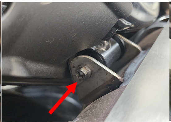
Fig.1.20 find screw holding muffer to mounting bracket and remove muffer.
