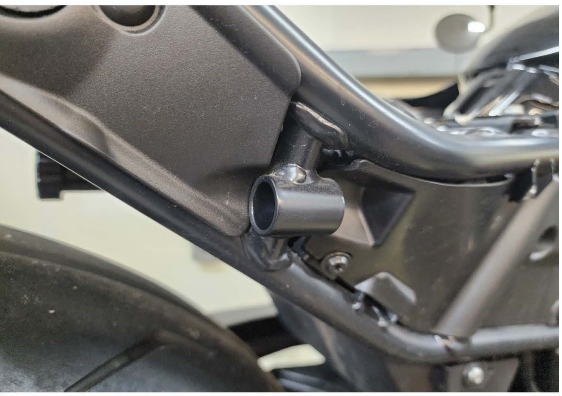
Fig.1.21 this is how the mounting bracket should look afterwards.
