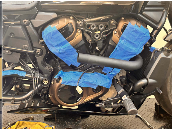
Fig.2.5 This is how it should look once finished (make sure to loosely tighten.)
