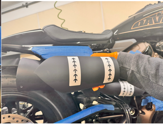
Fig.2.14 Grab the Apex heat-shield provided and insert worm clamps as shown to install
