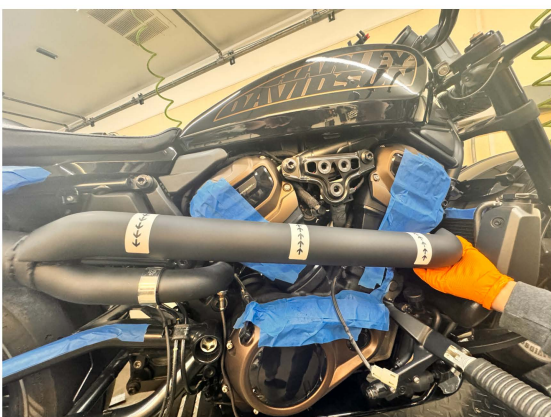
Fig.2.10 Grab the front heat-shield and insert worm clamps as shown above (do not tighten fully yet)
