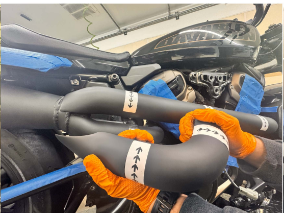
Fig.2.11 Grab the rear heat-shield and insert the worm clamps as shown above to install (do not tighten fully until both are on)
