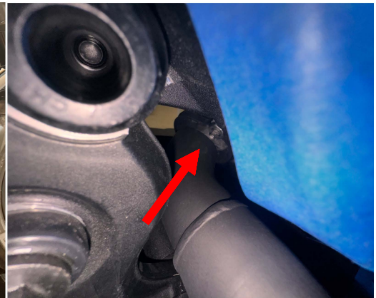
Fig.2.6 Insert the two screws for the rear pipe for installation as shown. Both pipes should face back.
