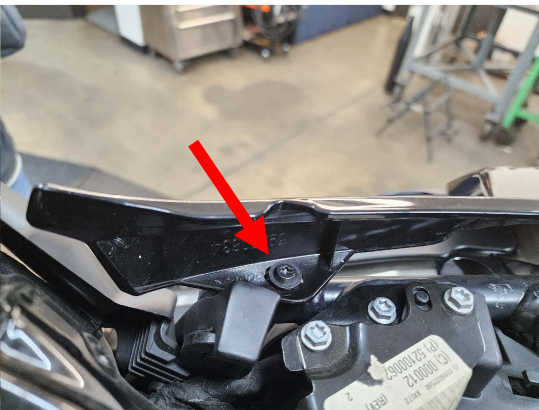
Fig.1.5 locate the front bolt holding down plastic cover and unscrew
