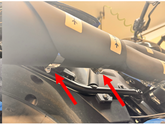
Fig.2.15 The worm clamps should look like this once put in the Apex heat-shield
