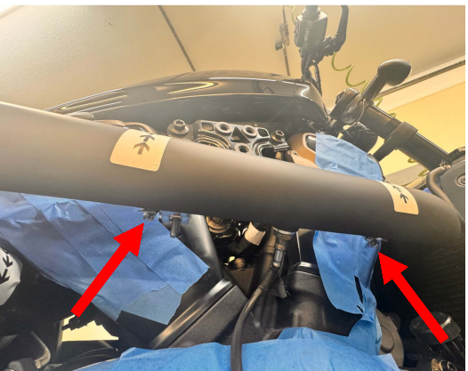
Fig.2.12 The worm clamps should look like this once put in the front heat-shield.
