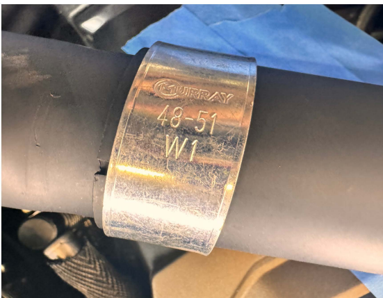
Fig.2.7 Connect the muffer into the head pipes as shown for both rear and front pipes with the clamp shown above.
