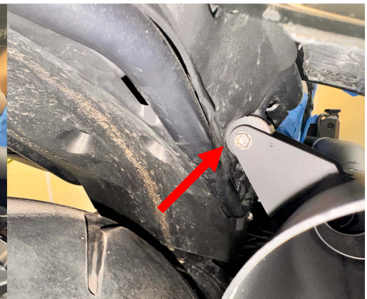
Fig.2.9 Align the muffer to the stock mounting bracket as shown and screw in (tighten all the headers and muffer clamps before putting on the heat-shields)
