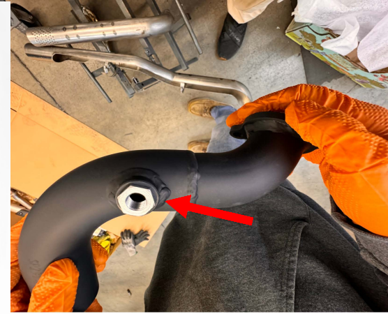
Fig.2.3 Insert the O2 sensor adapter into the O2 bung hole for both front and back head-pipes.
