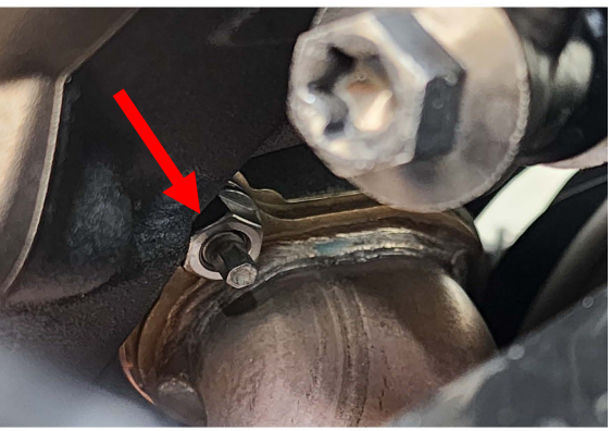
Fig.1.24 Locate the screws holding front header pipe to the engine and remove.
