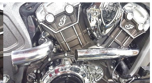
Fig. 2.5 install rear pipe
