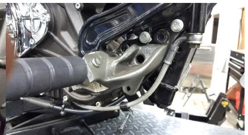
Fig. 2.20 install right control
