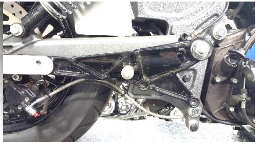
Fig.1.24 remove mounting bracket
