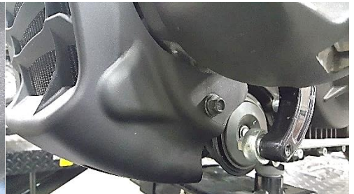
Fig. 1.9 remove screw left side
