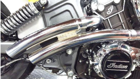
Fig. 2.9 install muffer assembly
