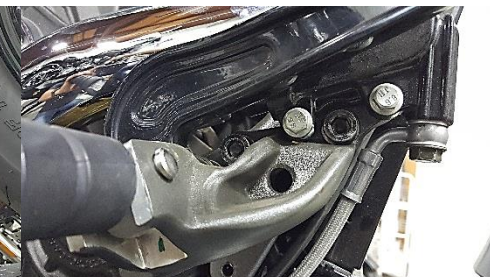
Fig. 1.11 remove right side control
