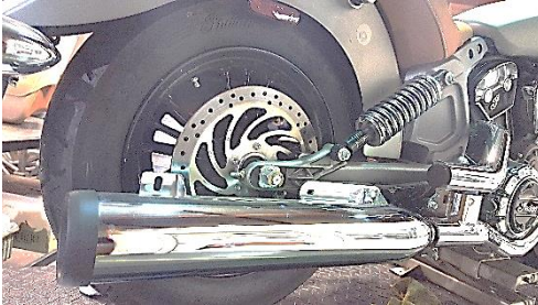
Fig. 1.4 remove top muffer
