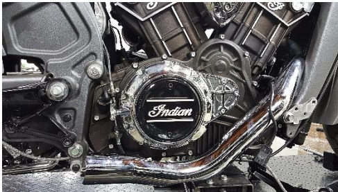
Fig. 1.22 remove rear pipe assembly
