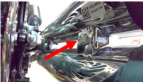
Fig. 1.1 remove muffer screw
