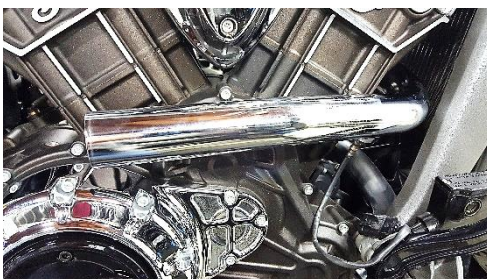
Fig. 2.3 install front pipe
