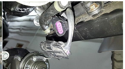
Fig. 1.18 disengage from harness
