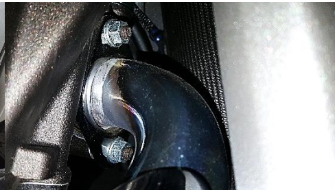
Fig.2.23 remove flange screw nuts
