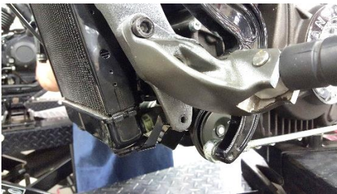
Fig. 2.21 install left control
