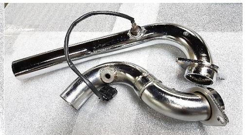
Fig. 2.2 install O2 sensor front pipe
