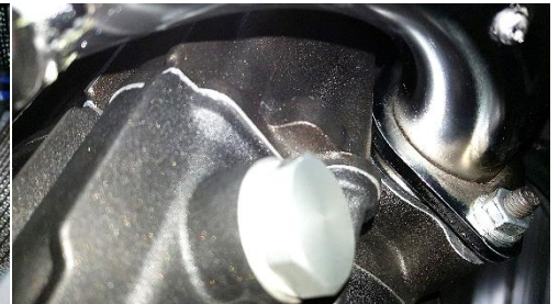
Fig. 2.14 tighten lower flange nut
