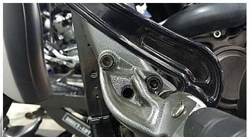
Fig. 1.12 remove left side control
