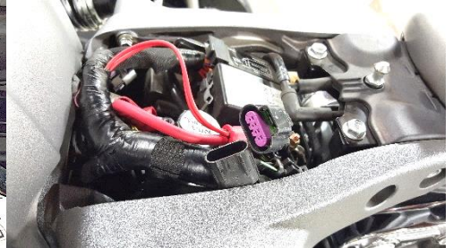
Fig. 1.6 disengage sensor harness
