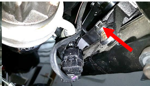
Fig. 1.17 don't cut plastic bracket
