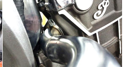
Fig. 2.11 tighten upper flange nut
