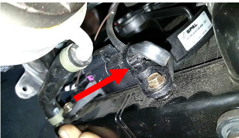
Fig. 1.16 cut off plastic zip tie
