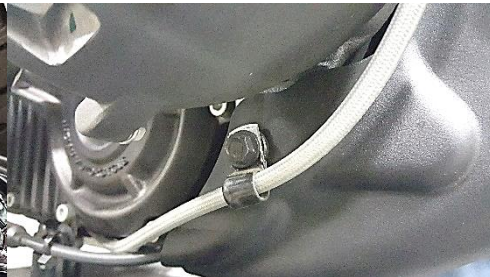
Fig. 2.8 remove screw right side
