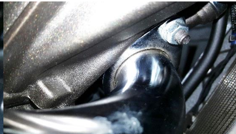
Fig.2.13 tighten upper flange nut
