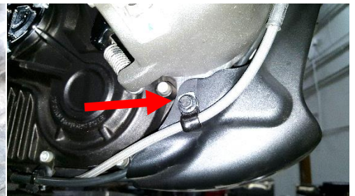
Fig. 2.23 install screw right side
