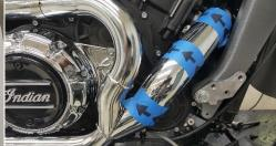
Fig. 2.14 place shield over pipe
