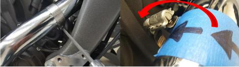
Fig. 2.15 tighten barrel clamp away from Fig. 2.16 install hose clamps heat shield.
