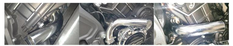
Fig. 2.3 install front pipe
