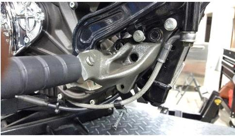
Fig. 2.21 install right control
