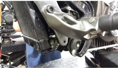
Fig. 2.22 install left control
