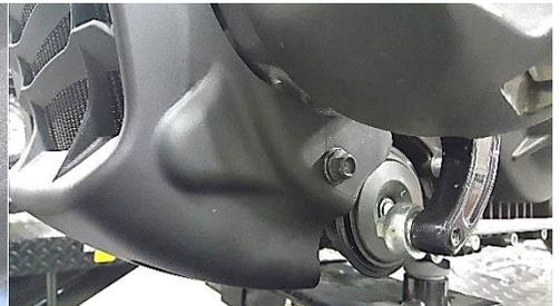
Fig. 1.9 remove screw left side
