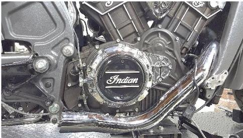
**Fig. 1.22 remove rear pipe assembly**
