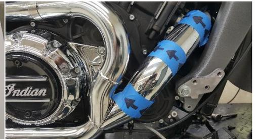
Fig. 2.14 place shield over pipe
