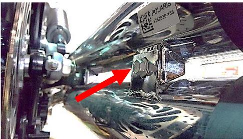
Fig. 1.1 remove muffer screw
