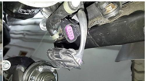
**Fig. 1.18 disengage from harness**
