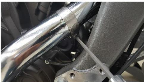
Fig. 2.15 tighten barrel clamp away from heat shield.
