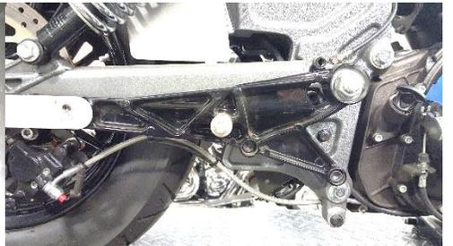
**Fig.1.24 remove mounting bracket**
