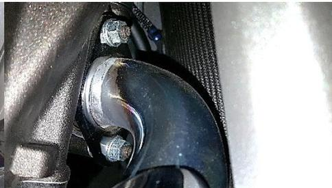
**Fig.2.23 remove flange screw nuts**
