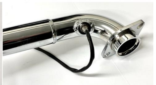
**Fig. 2.2 install O2 sensor front pipe**
