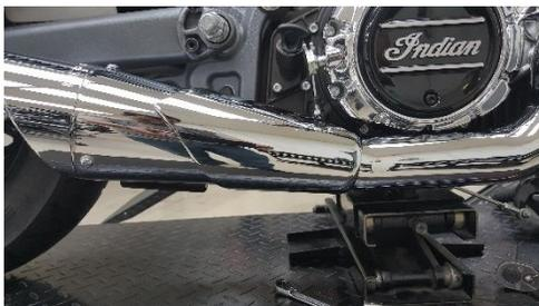
Fig. 2.18 install mid shield and megaphone shield
