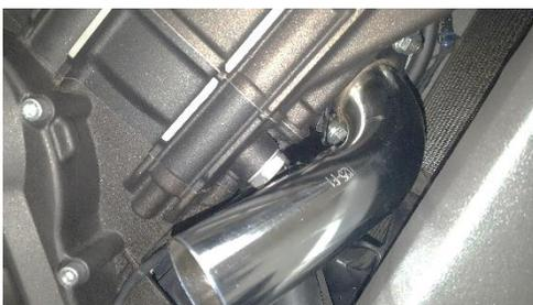
**Fig. 2.3 install front pipe**
