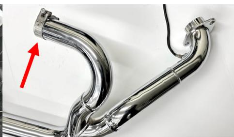
Fig. 2.7 insert clamp over inlets flush to edge
