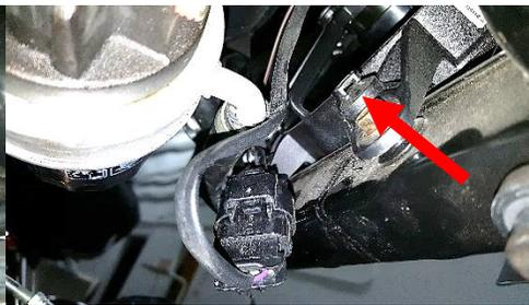
**Fig. 1.17 don't cut plastic bracket**
