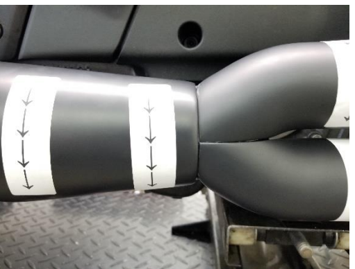
Figure 2.20 install muffler shield
