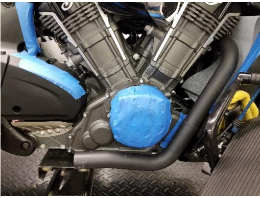
Figure 2.10 install front head pipe.
