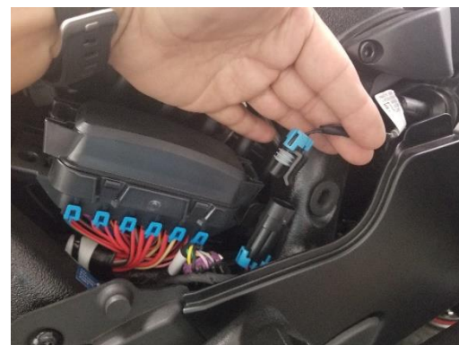
Figure 1.3 disconnect cable harness
