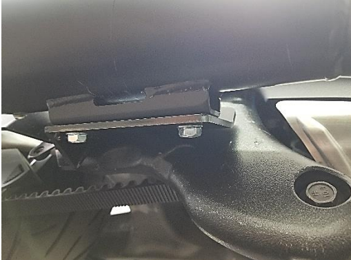
Figure 2.13 secure with screws and back plate
