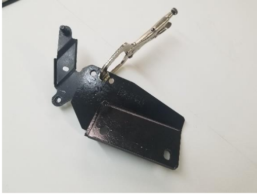
Figure 2.2 place new bracket over stock
