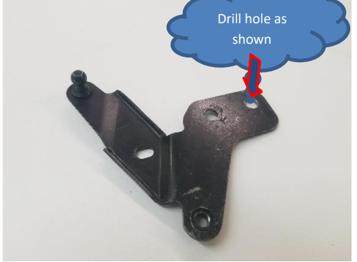
Figure 2.3 shown with hole drilled
