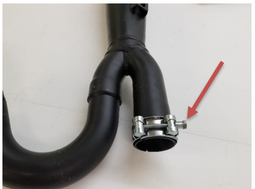
Figure 2.9 insert hose clamp arrow shows screw head
