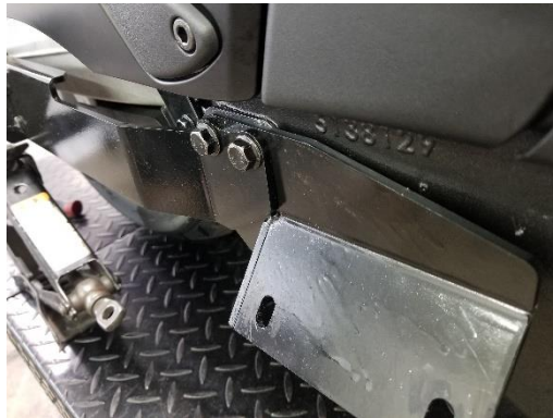
Figure 2.5 stock fist, system bracket second, saddle bag bracket last. Tighten brackets
