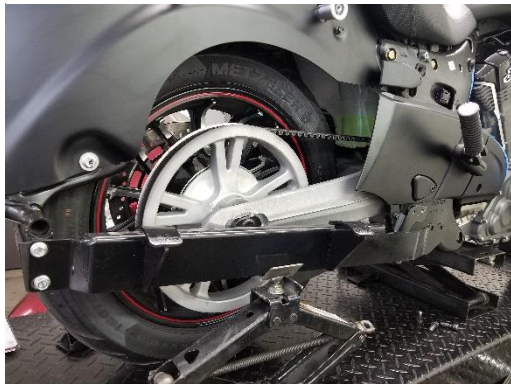
Figure 2.4 install right side bracket rear end first
