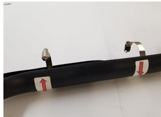
Figure 2.15 insert the first 2 front clamps front heat shield
