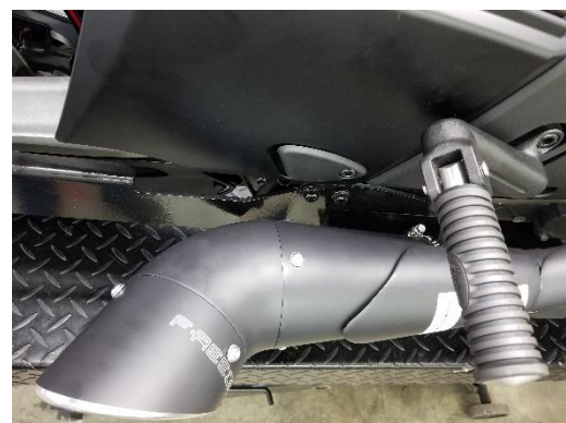
Figure 2.21 install end cap
