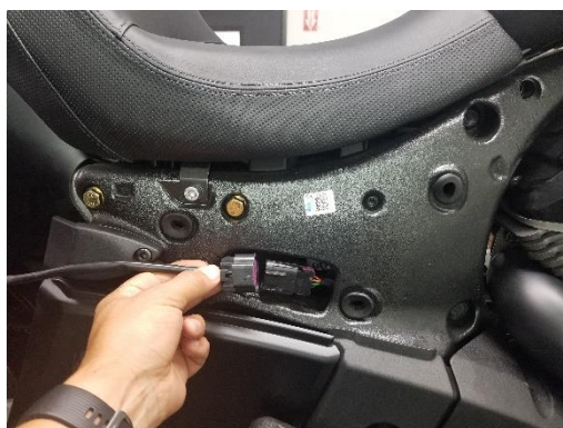
Figure 1.2 disconnect cable harness
