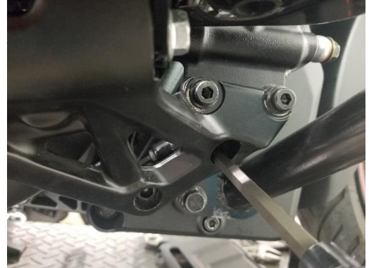
Figure 1.12 remove floorboard carefully
