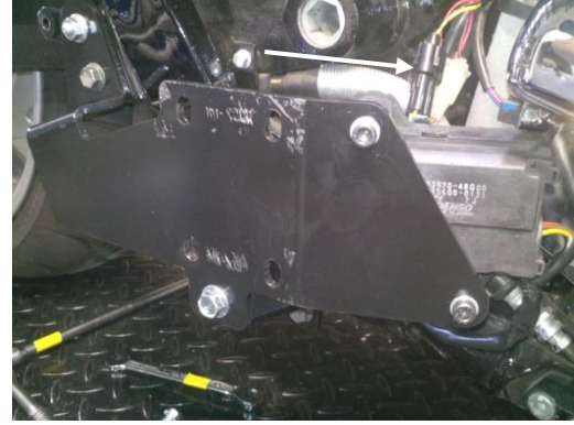
Figure 2.6 connect solenoid harness
