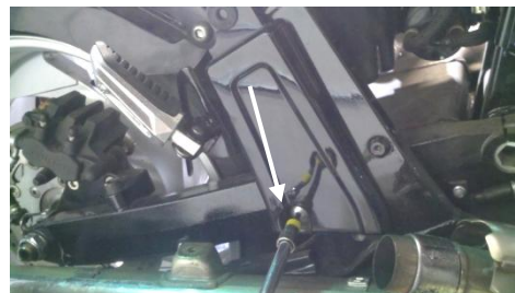
Figure 1.5 remove plastic cover (4mm)
