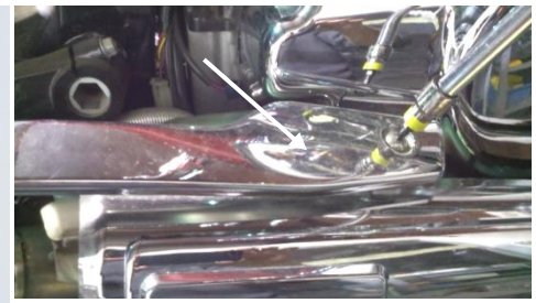
Figure 1.2 remove shield use 4mm allen
