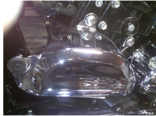
Figure 2.9 install chrome steel cover
