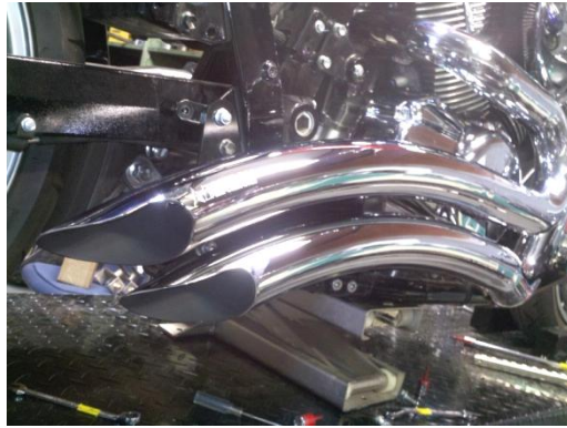
Figure 2.8 install rear pipe assembly
