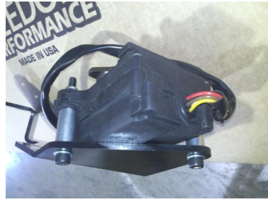
Figure 2.3 use 2 spacers 4 split washers 2 hex bolts and 2 nuts
