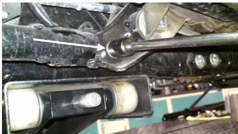
Figure 1.7 remove flange bolt 12mm
