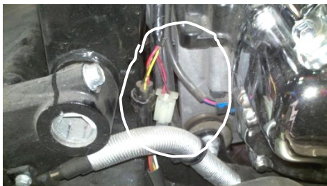
Figure 1.4 disconnect solenoid harness
