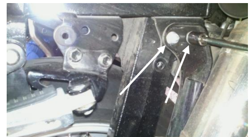
Figure 1.6 remove nut and bolt 12mm
