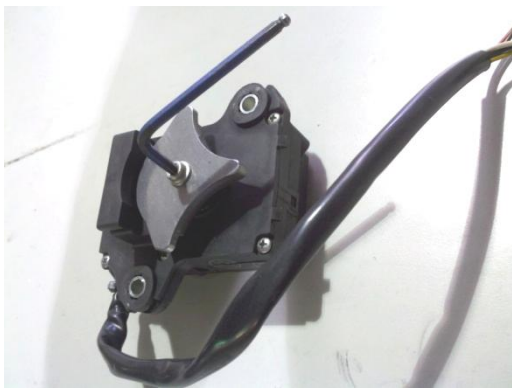
Figure 2.1 install cam as shown
