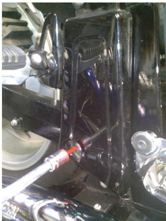
Figure 2.10 install plastic cover
