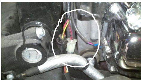
Figure 1.4 disconnect solenoid harness
