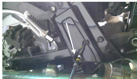
Figure 1.5 remove plastic cover (4mm)
