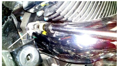
Figure 1.9 remove engine port bolts
