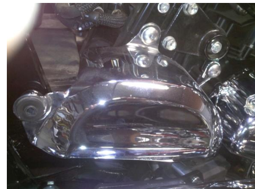
Figure 2.9 install chrome steel cover
