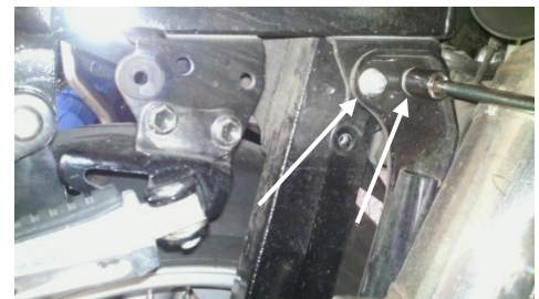
Figure 1.6 remove nut and bolt 12mm
