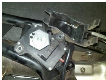
Fig 1.11 remove barrel end cables
