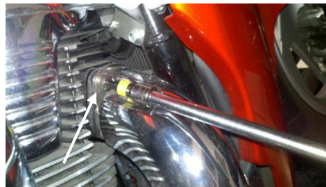
Figure 1.8 remove engine port bolts
