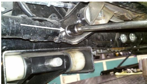
Figure 1.7 remove flange bolt 12mm
