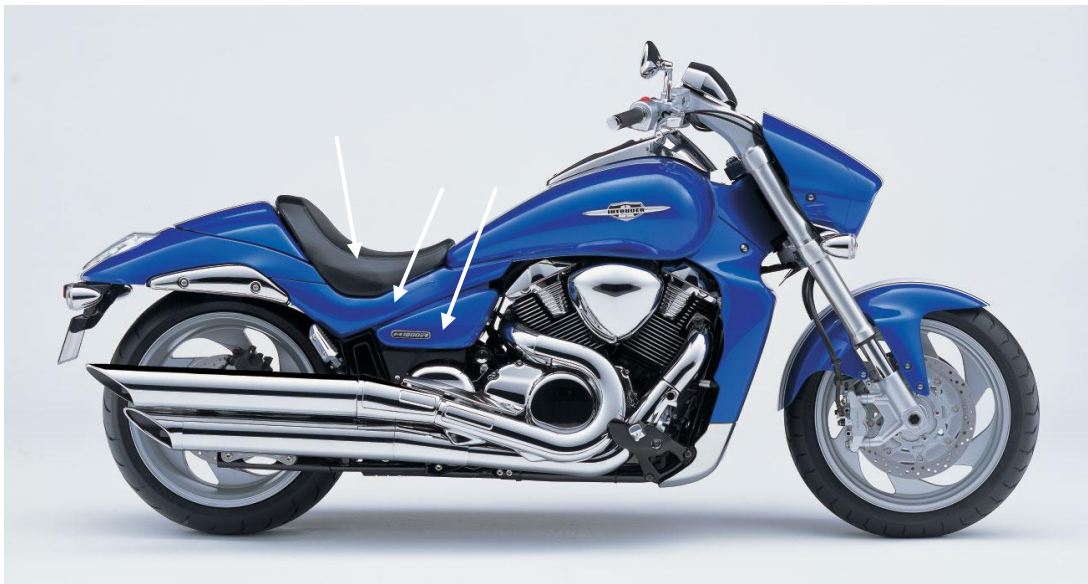
Figure 1.1 remove seat and side covers
