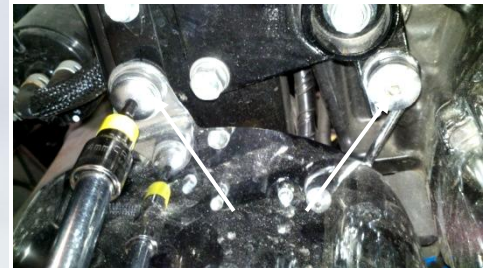
Figure 1.3 remove steel cover use 4mm
