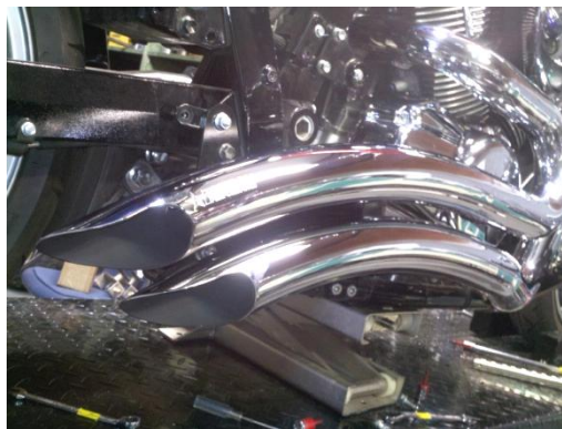
Figure 2.8 install rear pipe assembly
