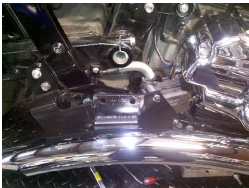
Figure 2.7 install front pipe assembly
