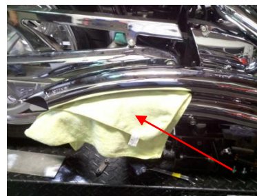
Fig 1.5 cover front shield gap and tighten to the mounting
