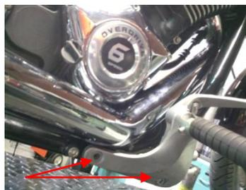
**Fig 1.1 remove peg assembly**
