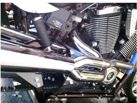
Fig 2.4 install muffler/header assembly
