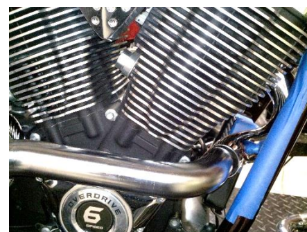
Fig 2.3 install front pipe with shield
