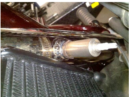
Fig 2.7 install sensor and connect to harness
