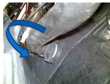
Fig 2.5 rotate hose if necessary away from rear header
