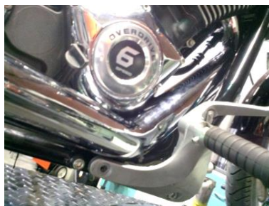
Fig 1.1 remove peg assembly
