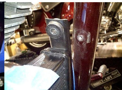
Fig 1.4 remove mounting bracket
