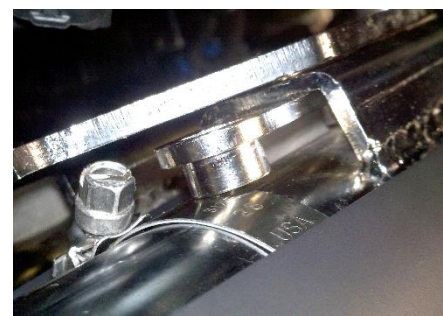
Fig 2.6 insert back plate bracket and secure it with two 5/16"-18 flange screws flat side seats against bracket
