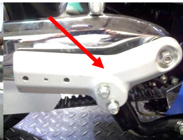
Fig 1.3 remove mounting bracket
