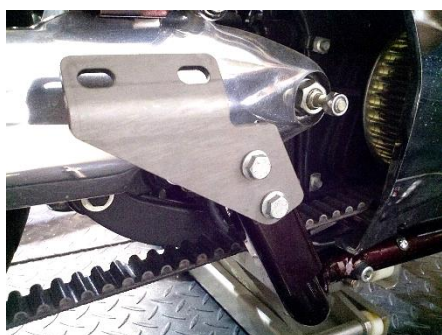
Fig 1.1 install mounting bracket (narrow frame shown)
