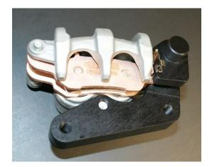
Always check your brake fluid level in your reservoir. New pads and rotors are thicker than the old ones and too much fluid in the system will not allow for expansion as the system heats up. This is a great time to bleed your brakes and even install Galfer stainless steel lines if not already equipped.
