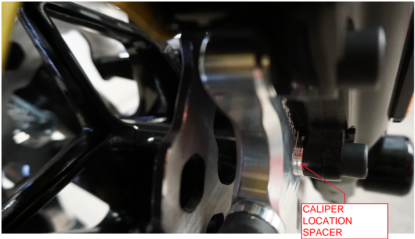
Picture #4 Bracket at Fork Mount
