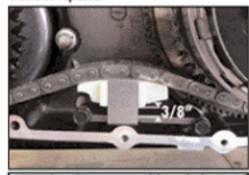
NOTE: The 3/8" is measured from the bottom of the shoe to the resting point of the springs on the guideplate, or shims.
