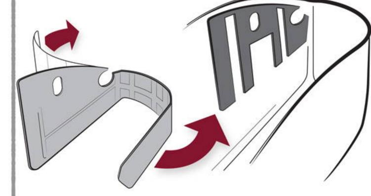
Peel adhesive back and place foundation over the top of the filler panel, and walk it around the inside of the saddle bag.
