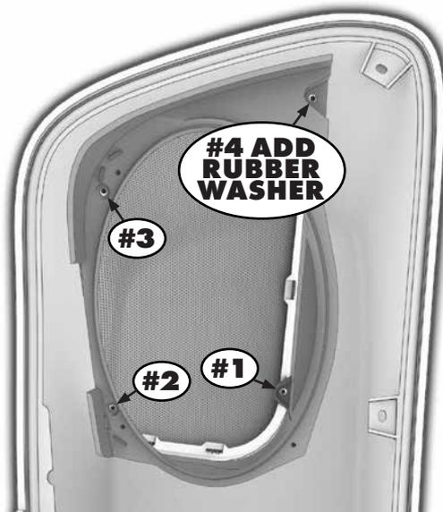
Have the lid upside down on a blanket or something similar to protect your painted surface. Locate the speaker adaptor marked "Brake" noting you will see it only fits one way. In the order shown, you will put "thread forming" screws through the adaptor and into the grill so the pieces "sandwich" the opening.
