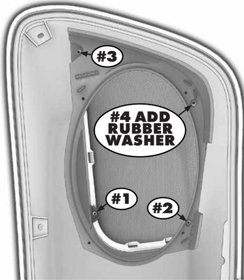
Have the lid upside down on a blanket or something similar to protect your painted surface. Locate the speaker adaptor marked "Clutch" noting you will see it only fits one way. In the order shown, you will put "thread forming" screws through the adaptor and into the grill so the pieces "sandwich" the opening.
