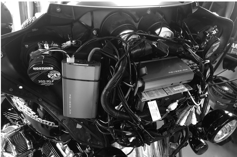
Showing the front speaker amp on top of radio and rear speaker amp mounted on 2CHSP Side Plate
