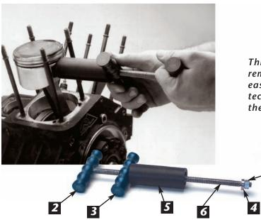
WRIST PIN REMOVER USE ON ALL MODELS INCLUDING TWIN CAM 88<sup>TM</sup>
