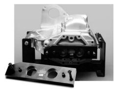
CAUTION: WEAR SAFETY GLASSES. EXCESSIVE FORCE MAY DAMAGE PARTS! SEE JIMS® CATALOG FOR OVER 100 OTHER TOP QUALITY PROFESSIONAL TOOLS. THE LAST TOOLS YOU WILL EVER NEED TO BUY. This tool will pull the complete trap door and gears from the transmission case, without damaging the door bearing, while leaving the main drive gear in the case.
