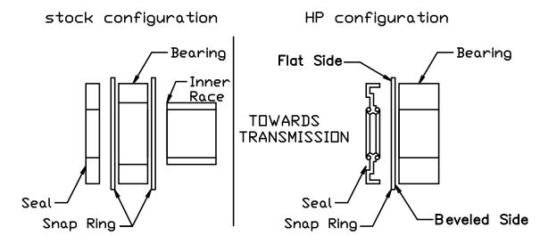
The outer snap ring is eliminated to accommodate the wider ball bearing.
