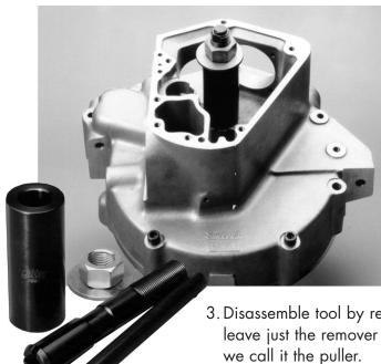
INNER CAM BEARING REMOVER USE ON BIG TWIN 1958-PRESENT SINGLE CAM ONLY. (NOTE: INCLUDES AFTERMARKET AND S&S® MOTORS
