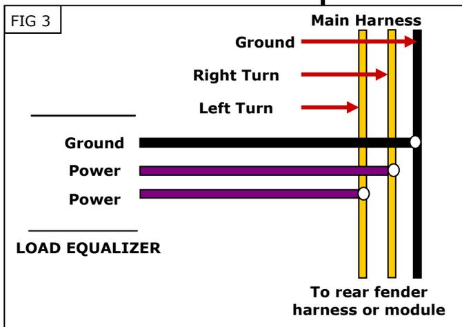
**CAUTION** Load equalizers generate heat when in use. Avoid using the turn signals for an extended period of time, otherwise the load equalizer will overheat. Never operate the four-way flashers unless you first remove the load equalizer. Overheating will damage the load equalizer, causing loss of turn signal operation and may create a fire hazard!
